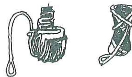
Wind rope-tail around bundle (two circuits makes it more secure) and tuck through itself
